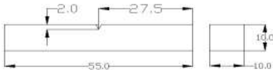
Charpy Impact test Specimen
