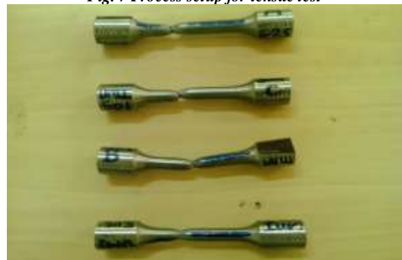
Fig. 8 Tensile test specimen after test
