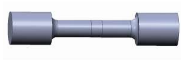
Fig. 15 Geometrical model of tensile specimen & butt joint in CREO
