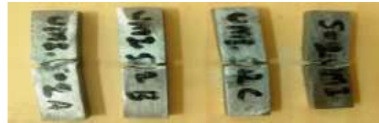
Fig. 11 Charpy impact test specimen after test
